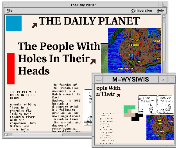
Figure 4: Multiple-WYSIWIS view. The main view at left shows the local user's view of the workspace; the inset window shows a remote participant's view.
